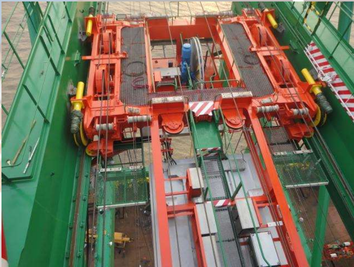
Trolley buffers on ZPMC cranes
